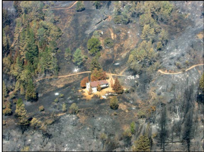
Figure 10.16. Long, narrow, one lane driveways with no turnouts can compromise ingress and egress and should be scouted before committing an engine to the assignment.
