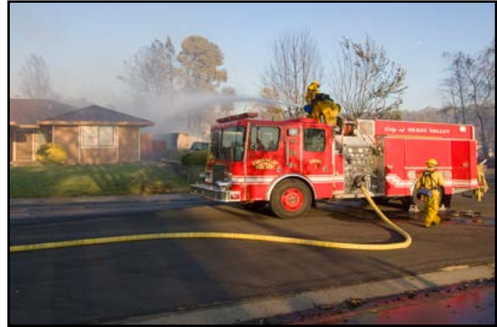
Figure 5.47. The Anchor and Hold tactic is well suited for engines capable of flowing large volumes of water with master stream devices.
