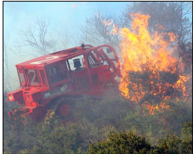
Figure 6.11. Dozers are best suited for direct and indirect control line construction over long distances.
