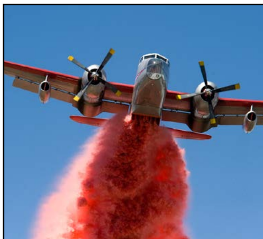
Figure 6.30. The payload of an air tanker includes the weight of the retardant and the velocity of the aircraft. Retardant drops have been known to cause tremendous damage to vehicles and structures as well as injuries to personnel on the ground.
