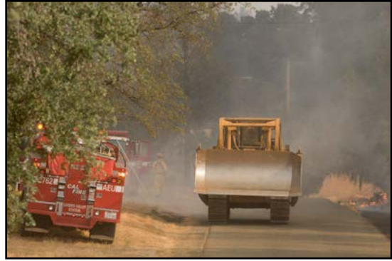
Figure 5.31. Dozers are an excellent tool to connect portions of secured control line, such as roads or driveways, to previously unsecured fire line when using the Connect the Dots tactic.
