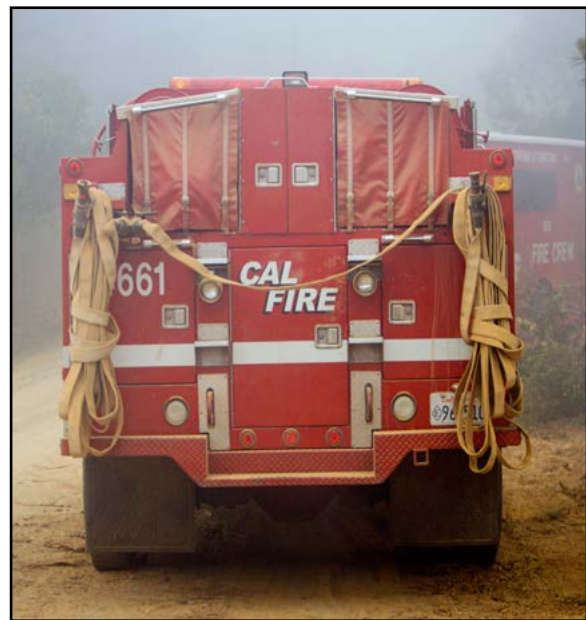
Figure 10.27. Engines traveling from structure to structure should secure hoses using WUI brackets to avoid dropping or dragging hose along the roadway.
