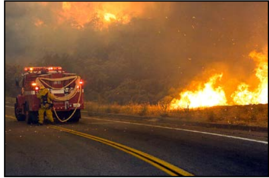
Figure 5.28. WUI hose brackets allow for the rapid deployment of hose during the Bump and Run tactic. The brackets allow for the secure stowing of the hose when the engine is ready to advance.
