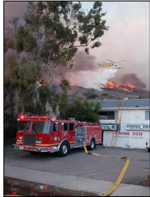
Figure 5.42. Engines using the Prep and Defend tactic should back into position, ladder the roof for debris removal, provide a water source to the engine from the structure, and concentrate preparation efforts on the fire impact side of the structure.
