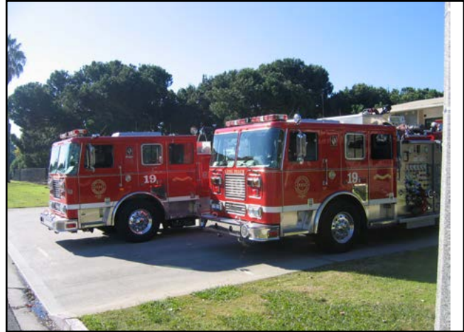
Figure 6.1. Type 1 and Type 2 engines, though not usually outfitted for WUI incidents, play an important role in structure defense and perimeter control.
