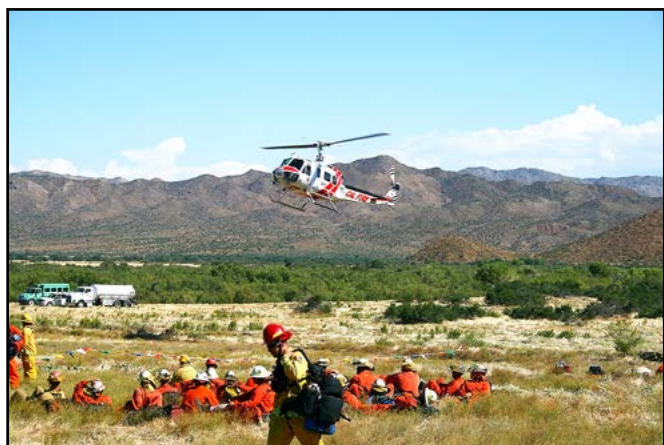
Figure 6.17. The versatile Type 2 helicopter not only performs direct suppression tactics such as water drops, but also performs support missions such as crew shuttles and cargo deliveries.
